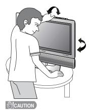
Adjust the screen with both hands. Put one hand on the Display and tilt the screen while steadying the stand with your other hand.
